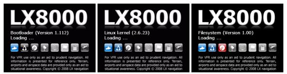
The boot procedure normally takes 30 seconds but in the case of a firmware update or system check it can take more time. On the last boot screen information about LX8000 firmware and IGC serial number is shown.
